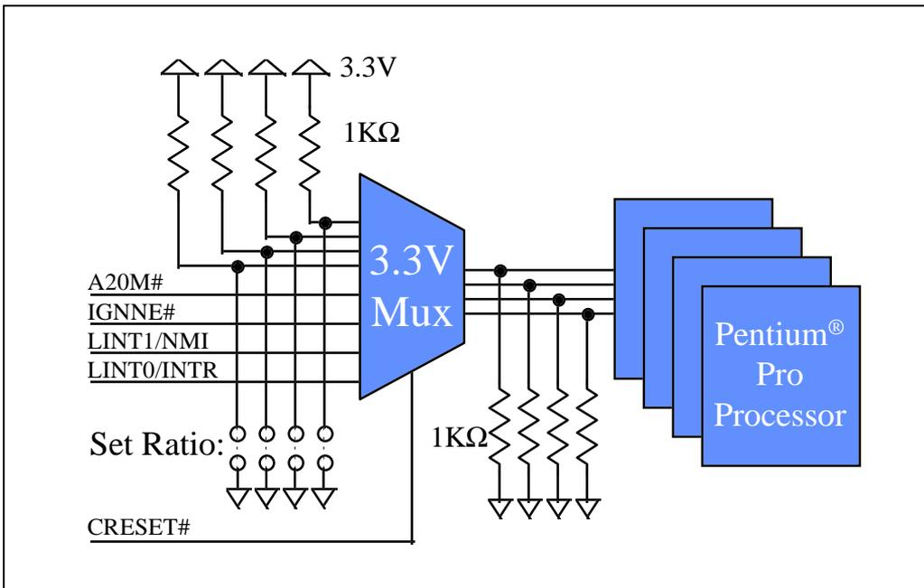
Figure 11-4. Example Schematic for Clock Ratio Pin Sharing
