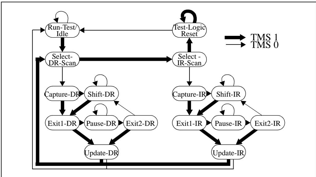
Figure 10-2. TAP Controller Finite State Machine
