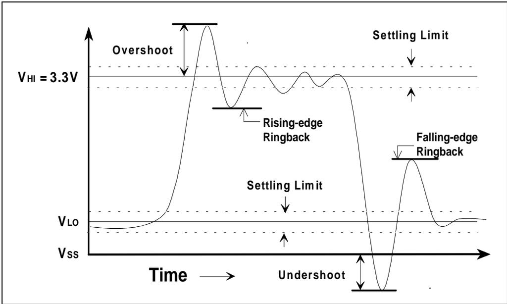
Figure 13-1. 3.3V Tolerant Signal Overshoot/Undershoot and Ringback
