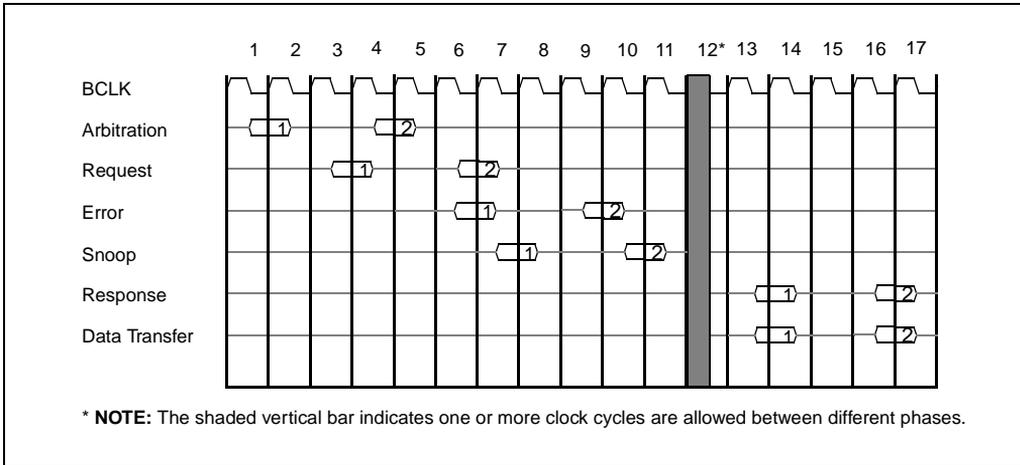
**Figure 3-2. Pentium® Pro Processor Bus Transaction Phases**
