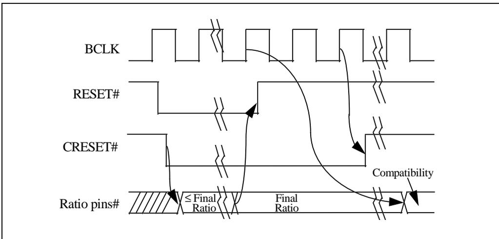
Figure 11-3. Timing Diagram of Clock Ratio Signals
