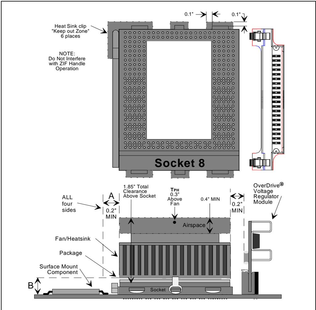
Figure 17-4. Space Requirements for the OverDrive® Processor
