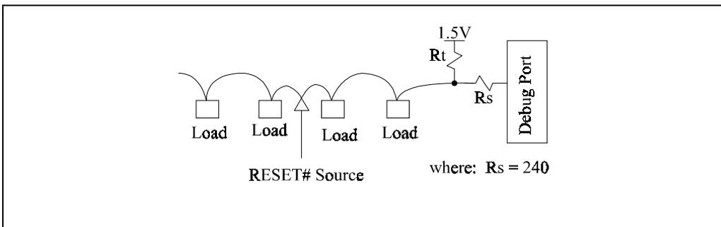
**Figure 16-1. GTL+ Signal Termination**
