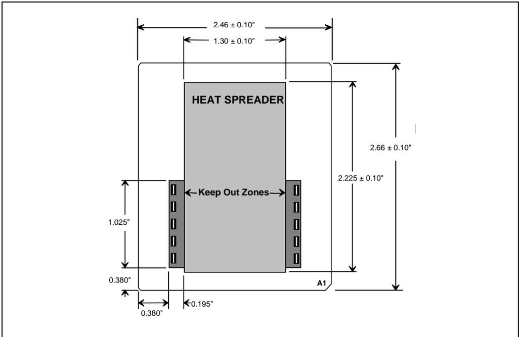
Figure 15-2. Top View of Keep Out Zones and Heat Spreader
