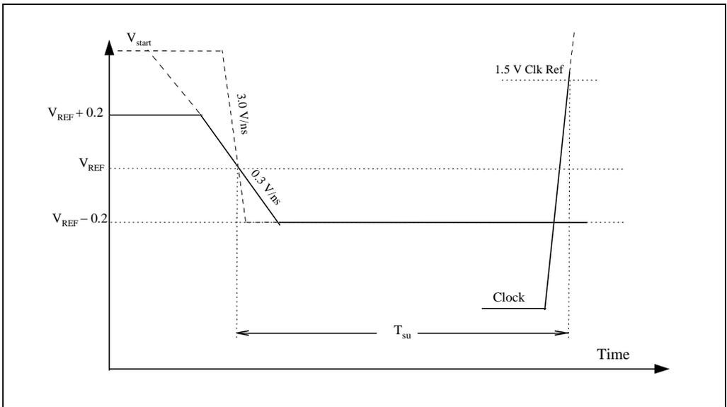
Figure 12-14. Standard Input Hi-to-Lo Waveform for Characterizing Receiver Setup Time
