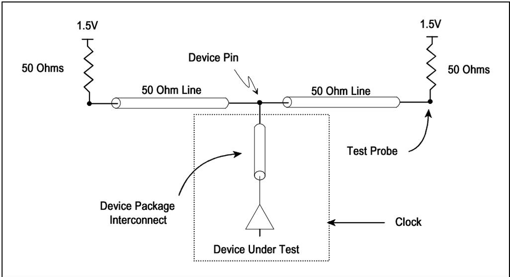
Figure 12-11. Test Load for Measuring Output AC Timings
