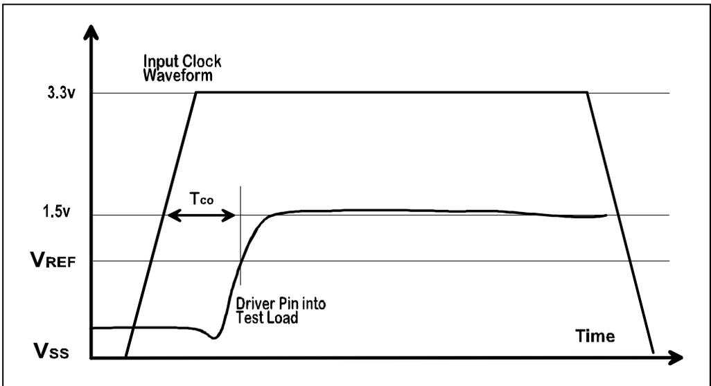
Figure 12-12. Clock to Output Data Timing ( $T_{CO}$ )
