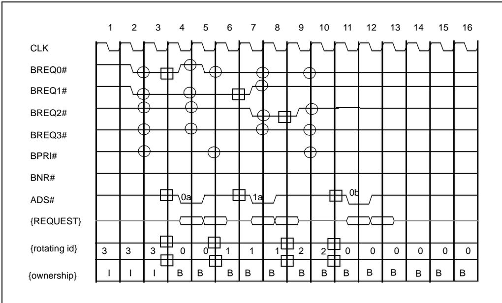
Figure 4-6. Symmetric Arbitration with no Transaction Generation
