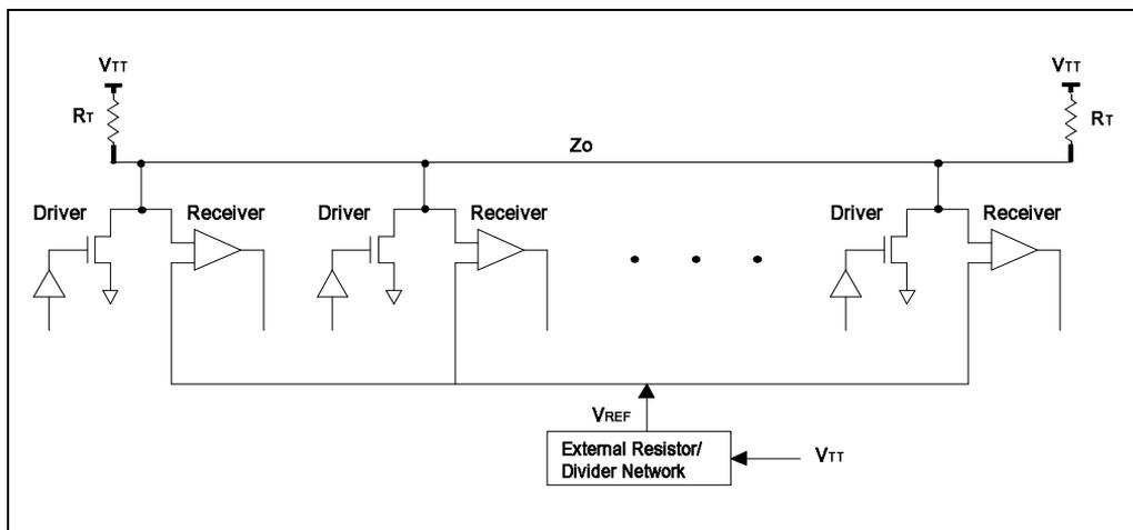
Figure 12-1. Example Terminated Bus with GTL+ Transceivers
