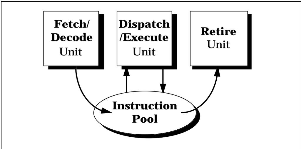
Figure 2-1. Three Engines Communicating Using an Instruction Pool
