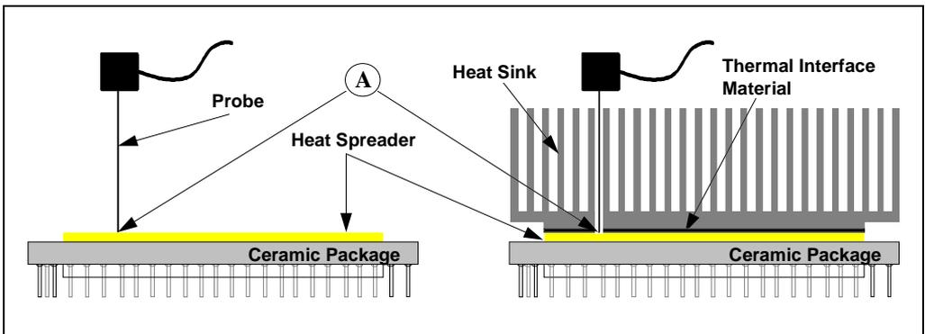
Figure 14-2. Thermocouple Placement
