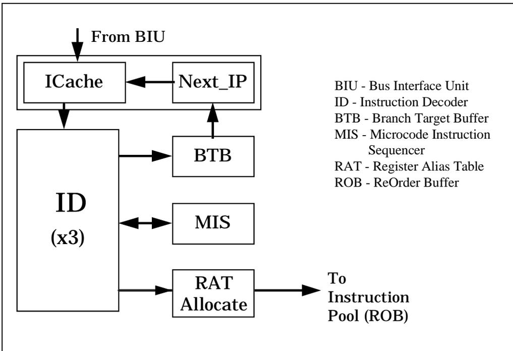
Figure 2-4. Inside the Fetch/Decode Unit
