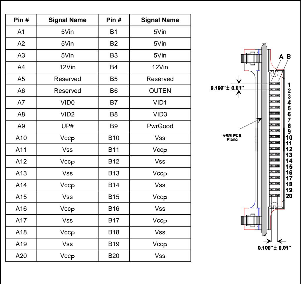
Figure 17-5. Header 8 Pinout
