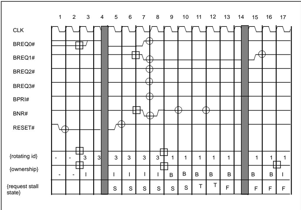
Figure 4-4. Delay of Transaction Generation After Reset
