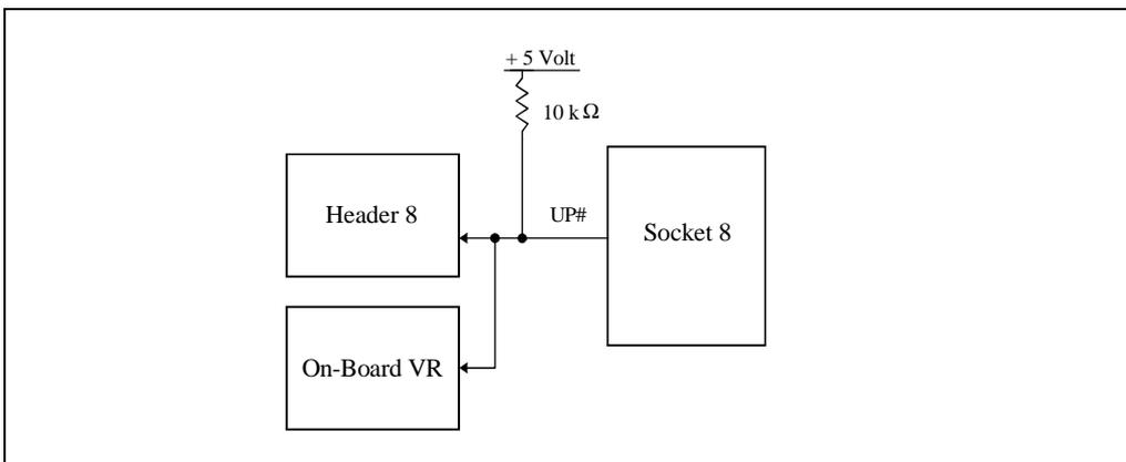
Figure 17-8. Upgrade Presence Detect Schematic - Case 2
