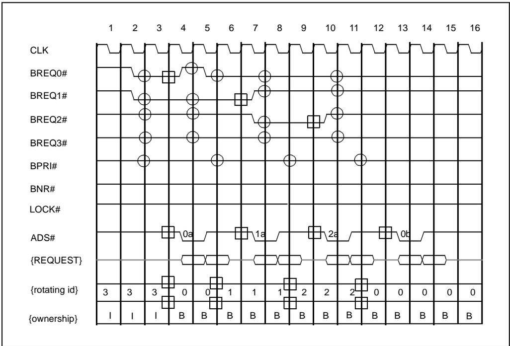
**Figure 4-5. Symmetric Bus Arbitration with no LOCK#**
