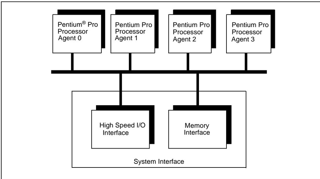
Figure 1-2. Pentium® Pro Processor System Interface Block Diagram
