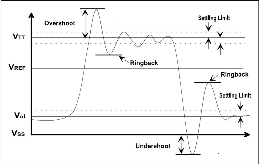
Figure 12-2. Receiver Waveform Showing Signal Quality Parameters
