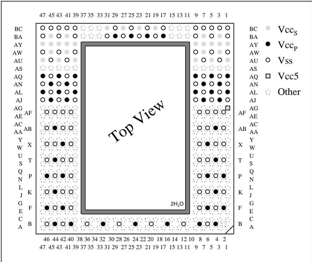
Figure 15-3. Pentium® Pro Processor Top View with Power Pin Locations
