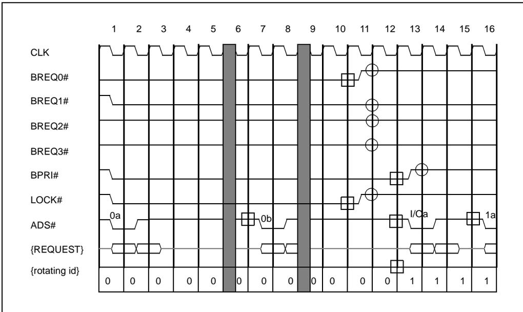
**Figure 4-8. Symmetric and Priority Bus Exchange During LOCK#**
