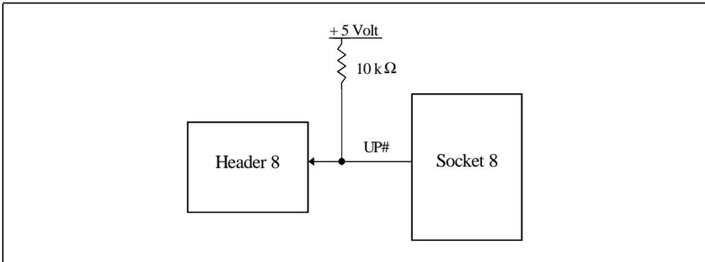
Figure 17-7. Upgrade Presence Detect Schematic - Case 1
