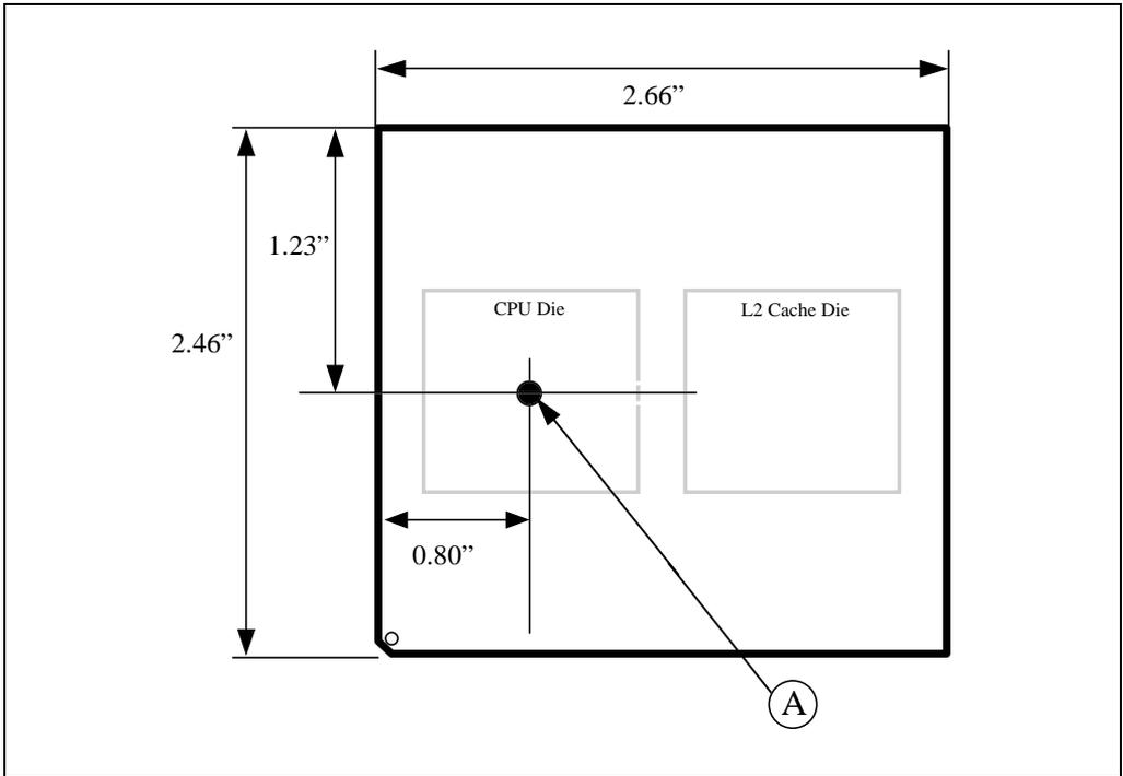
Figure 14-1. Location of Case Temperature Measurement (Top-Side View)
