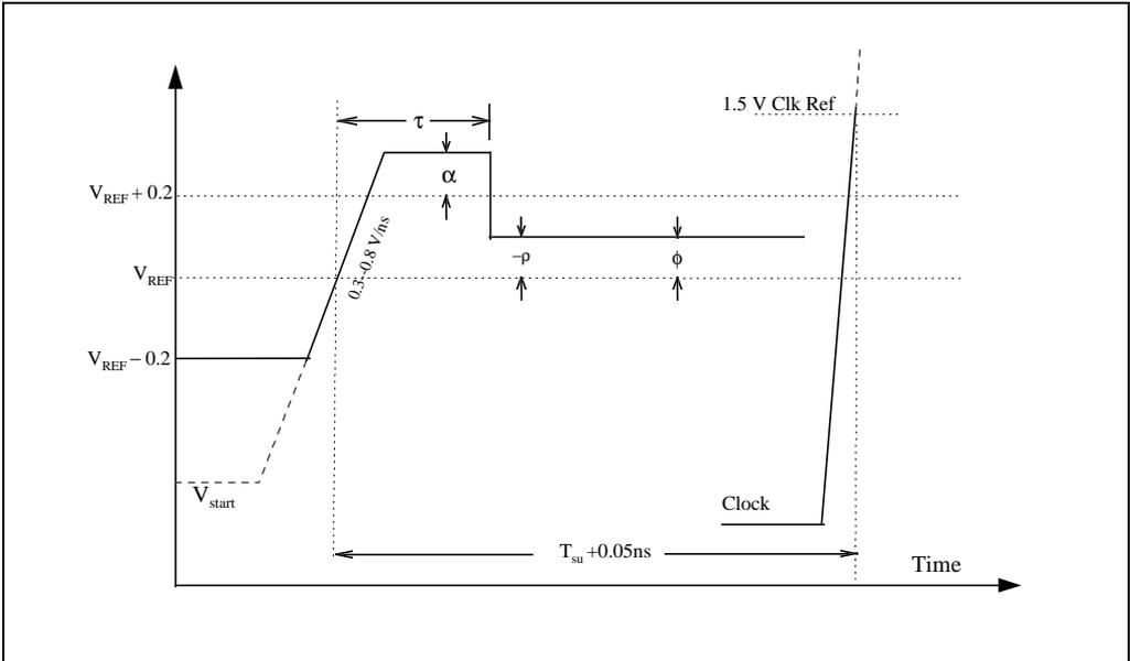
Figure 11-10. Lo to Hi GTL+ Receiver Ringback Tolerance
